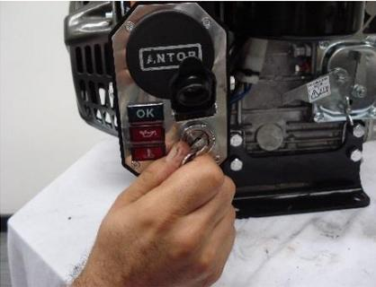
18. Turn the engine switch clockwise to the ON position. Warning lights will light.
